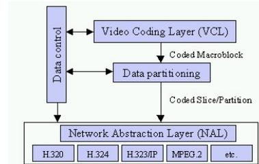
Fig. 1. H.264 / MPEG-4 AVC layer structure.
