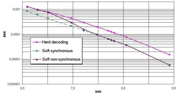
Fig. 4. Decoding results in terms of BER for 'Foreman' first I frame.
