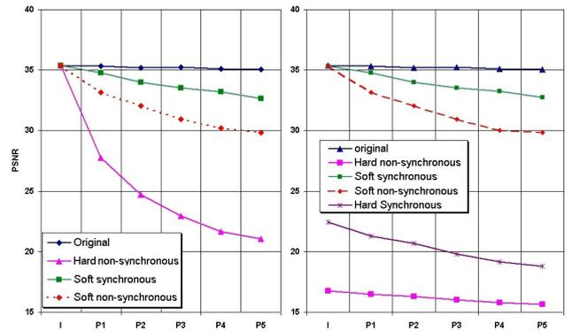
Fig. 7. Decoding results in terms of PSNR for beginning of 'Foreman' video sequence (IPPPPP), with noise-free or noised I slice.
