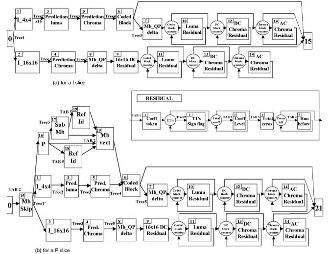
Fig. 3. A Macroblock decoding process for both I or P slices.
