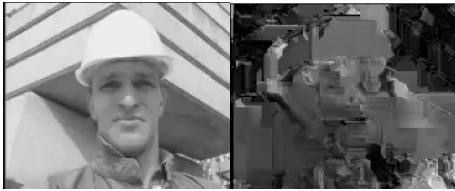
Figure 4 - Visual results for de-ciphered and ciphered 1 st frame of 'Foreman' sequence (I coded), QCIF format, QP=30.
