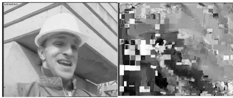
Figure 5 - Visual results for de-ciphered and ciphered 115 th frame of 'Foreman' sequence (P coded), CIF format, QP=30.
